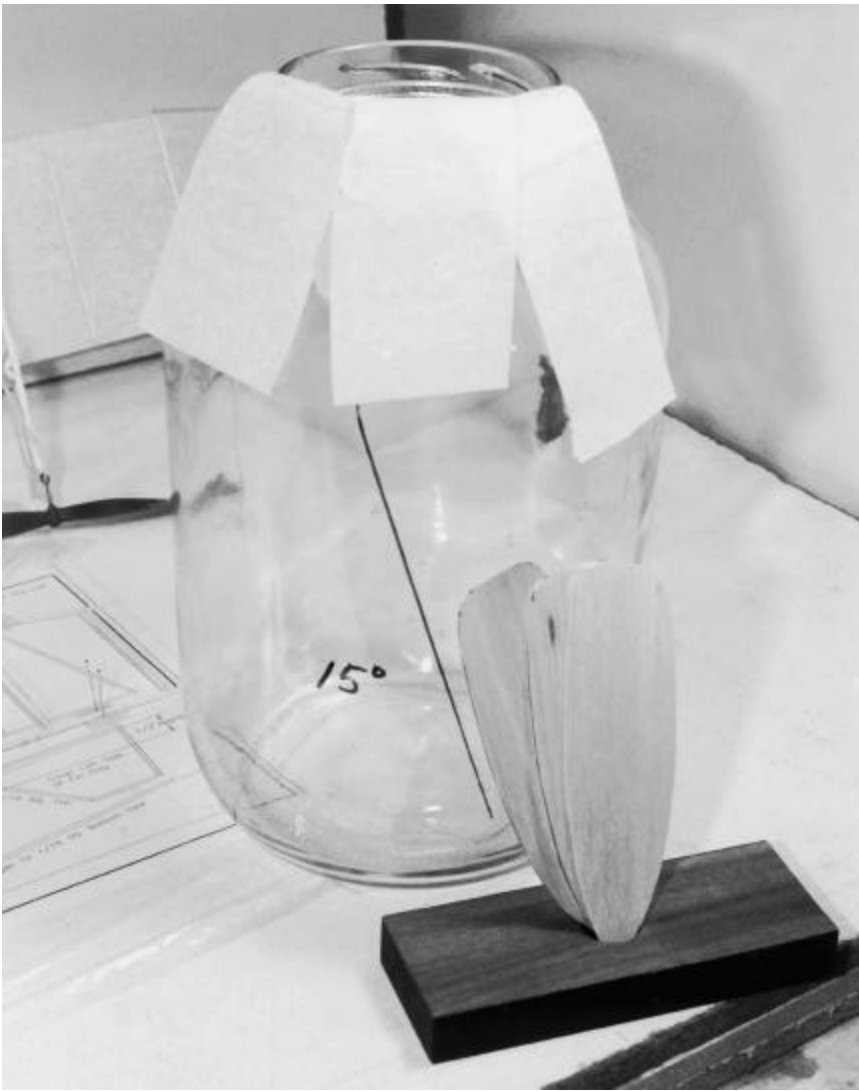
Three blades and tissue ready to soak/stack/bake on six-inch diameter jar. Blades angled 15° to impart pitch
